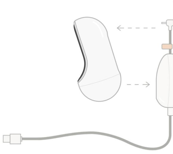
Attach the Owlet Cam 2 to the magnetic base. Plug the cable into the Owlet Cam 2.
